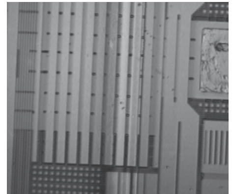
20X NIR confocal image of CIS device (front)
